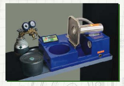
The microprozessor- and sensor controled machine is computing individually the lowest gas consumption for each preservation according to the content of the printing-ink box. Operating of the machine is mostly simple: The preservating printing-ink box is placed into the machine and the seal has to be set in. Preservation starts automatically after closing the lid and pressing the start key. No more working step is necessary.
